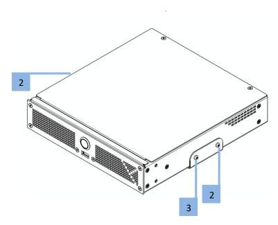
2. Use M3 Screws to attach the PXm to the VESA mount, there are two holes either side for a total of four screws.
