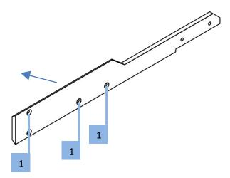
1. Attach the male centre section to the inside face (right) of the unit to be mounted on the left-hand side (looking at the rack from the front), using four countersunk M3 screws.
