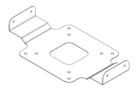
1. Attach VESA mount to rear of screen with the tabs at the top and bottom.
