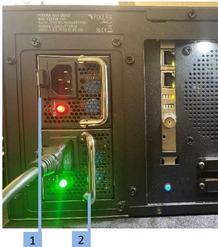
1. Push the release tab on the back of the power supply.
