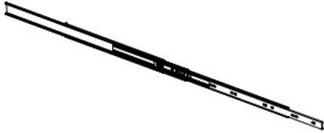
2. Place the front bracket on the outer rail. Set the first hole of the outer rail to the sixth hole of the bracket and screw the bracket to the rail.
