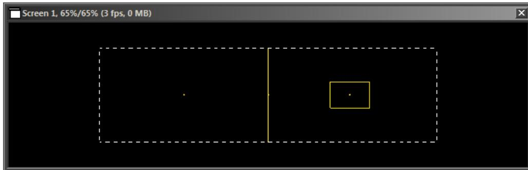
Apply this screen field to a track. Now the content on this track is scaled and placed on the right side, it fits the screen field.
