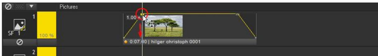
The figure shows that the second node was moved downwards. The brightness changed from 100% to 54.7% now. The current value of the selected node is shown next to it (except the value is 100%).
