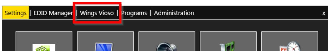
In the Wings Vioso tab, the check box next to "Use Wings RX" needs to be selected (it is preselected on all RAW Engines).
